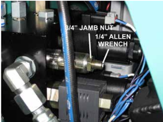
Figure 29. Pitch Pressure Adjustment
